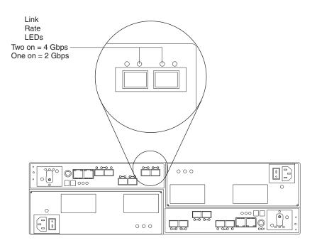
Figure 81. Link rate LEDs
